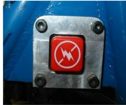
The machined block constraining the switch
