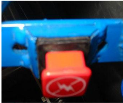
The welded metal tabs constraining the switch
